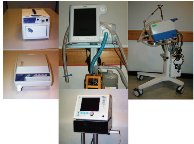
Fig. 10. Current commercially available noninvasive ventilators. Clockwise from upper left: Respicronics STD30, Respicronics V60, Dräger Carina, Respicronics Vision, Sullivan VPAP.
